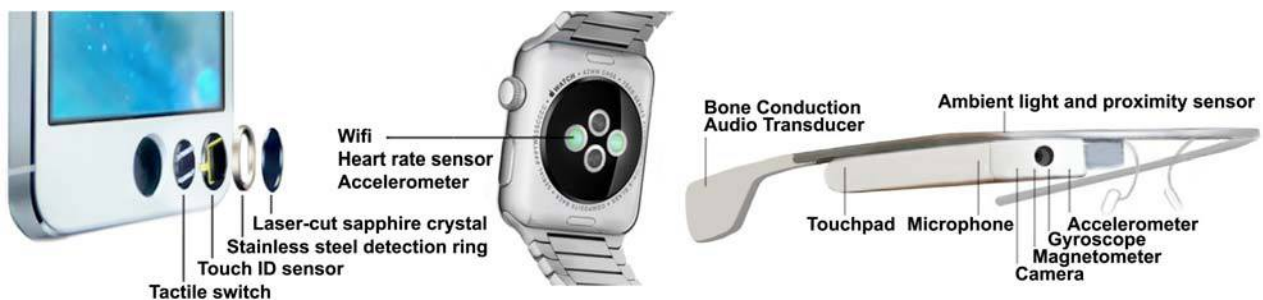
Fig. 12 Sensor integration with the purpose of facilitating rich interactions.
