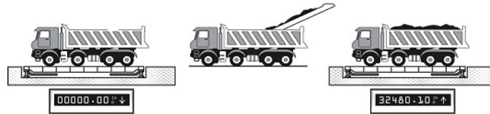
Figure 5: Computing in real time the volume of coal extracted. The weight can also be easily established.
