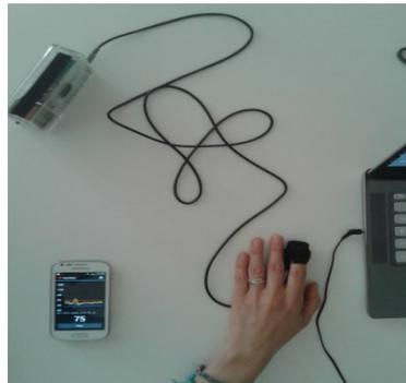
Figure 4: Image of the CardioAlert prototype. On top left, the heart rate recorder that receives the changes in the hemoglobin detected by a led sensor connected to an individual's finger. This signal is filtered, amplified and elaborated to obtain the heart rate by using an Arduino microcontroller. On bottom left, is the smartphone which receives the data from the microcontroller by a Bluetooth connection.
